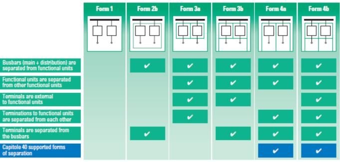
Internal separation in accordance with IEC 60439-1
